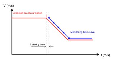
When activating this SLS, the parameterized SSX is automatically activated via the SLS. The SSX now monitors the ramp course of the speed. If the actual speed is lower than the SLS threshold, the SLS will take over the further monitoring, until the SLS is deactivated again.
