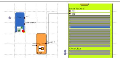
*Note*: When editing the associated inPort element, the connection with the start element is deleted and cannot be restored automatically. It must subsequently be supplemented manually.
