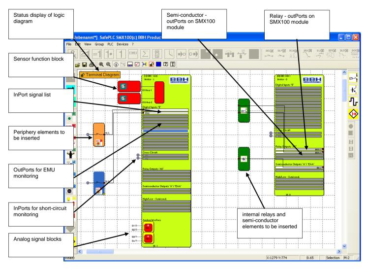
If function blocks are inserted into the terminal diagram, the elements will automatically be wired. In some instances it may happen, that the connections are unfavourably displayed. This, however, <u>has no adverse effect on the functionality</u>. You can trigger redrawing of the connection by displacing then corresponding block. Existing connections can also be erased and subsequently generated by hand.
