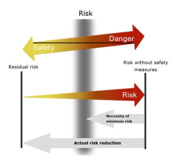
The risk analysis must account for all operating conditions of the machine, such as operation, setup work and maintenance or installation and decommissioning as well as predictable erroneous operation.
