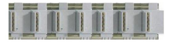
There is no TB2 between the last SMX11 module and the communication module SMX5x because the power supply for the SMX5x is fed in through the backplane bus system.
