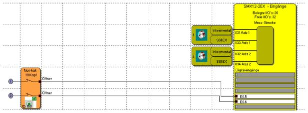
Emergency stop contacts from emergency stop relay with pulsing from the SMX
