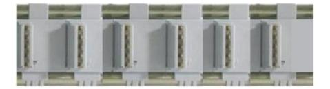
There is no TB2 between the last SMX121-2 module and the communication module SMX5x because the power supply for the SMX5x is fed in through the backplane bus system.
