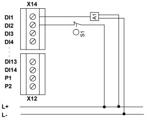
Figure: dual-channel input element heterogeneous, without cycling
