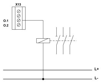
Fig.: Wiring of a auxiliary output
