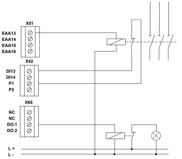
Fig.: Two-channel output with single-channel wiring with testing
