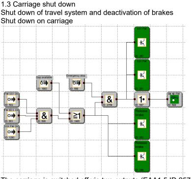
The carriage is switched off via two outputs (EAA1.5 ID 257 and 1.6 ID 261). The brakes are released via two outputs (EAA1.3 ID 253 and 1.4 ID 249). The PLC receives a message concerning bit 40 (ID 600). In case of an emergency stop the shut-down takes place immediately.
