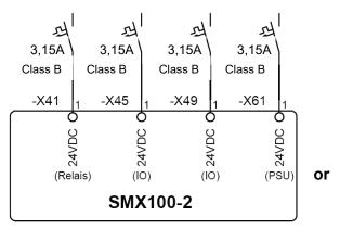
Connection example with separate IO supply! (when connecting IO's with high current consumption)
