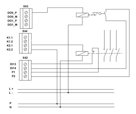
4.3.4.2.6 Dual-channel output with relay output and external control circuit in PI e
