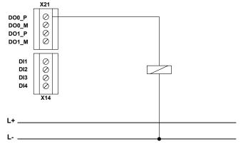
Fig.: Single-channel switching P-output.
