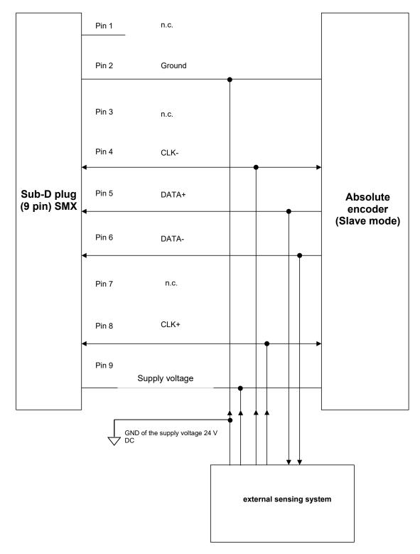
With this type of connection both clock signals and data are read in. In this example the module does not supply the encoder with voltage.
