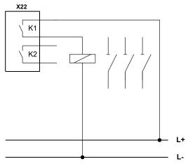
Fig.: Single-channel switching relay output.
