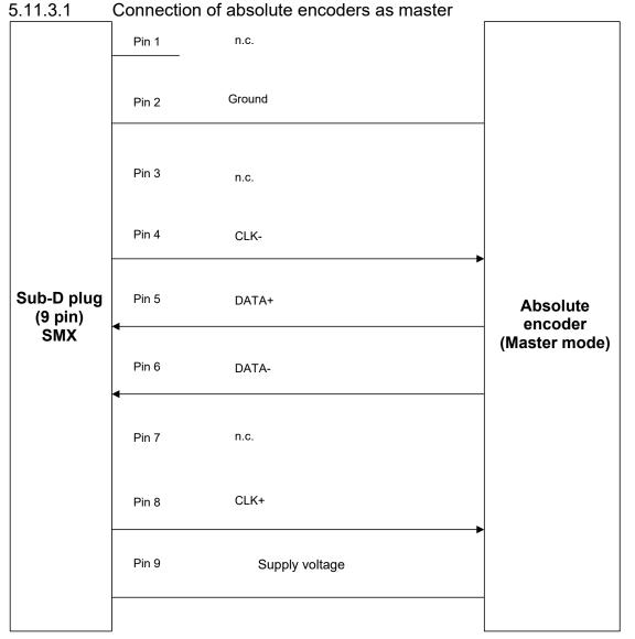
With this type of the connection the clock pulses of the module SMX100 run to the absolute encoder and the data from the encoder to the SMX100.
