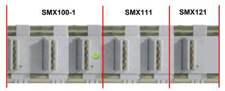
There is no TB2 between the SMX111 module and the communication module SMX121 because the power supply for the SMX121 is fed in through the backplane bus system.
