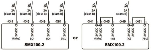
Connection example with separate I/O supply! (when connecting I/Os with high power consumption) Connection example with common I/O supply! (when connecting I/Os with low power consumption)
