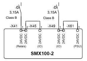
Connection example with bridged IO supply! (when connecting IO's with high current consumption)
