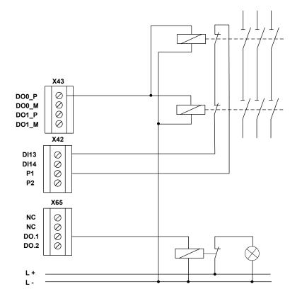
*Fig.:* Single-channel switching outout DO0\_P with dual-channel external circuit and monitoring at input 1 as group feedback
