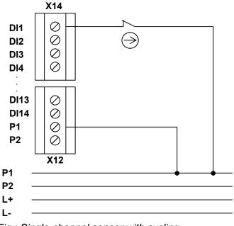
Fig.: Single-channel sensor with cycling
