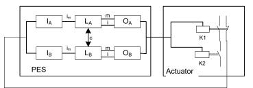
Single-channel output SMX with internal dual-channel processing (EAAx) and dual-channel actuator with at least single-channel diagnose
