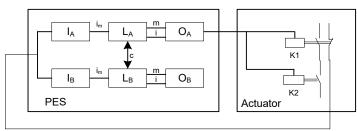
Single-channel output SMX (Rel 1 / 2, DO 0/1P, DO 0/1M) and dual-channel actuator with at least single-channel diagnostics.
