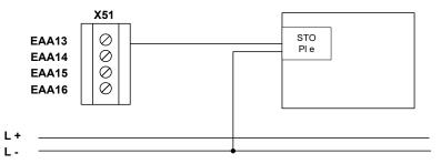
Fig.: Two-channel output in connection with a device with with examined disconnection
