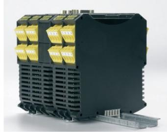
Snap the backplane bus element into the C-rail and insert it into the counter-piece by sliding it sideways.
