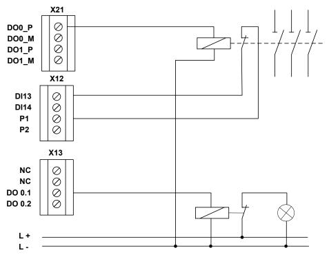
Fig.: Single-channel relay output with testing
