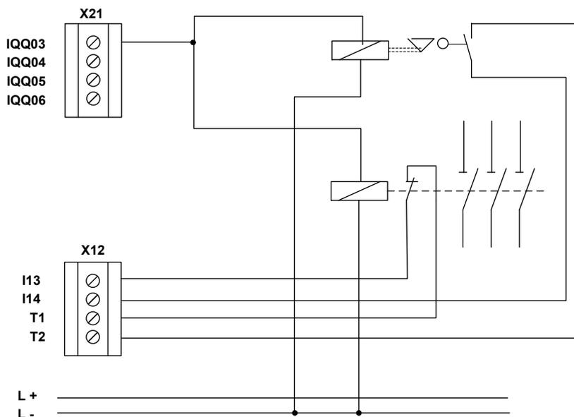
**Fig. 29: Dual-channel output in conjunction with dual-channel switch-off circuit with testing**
