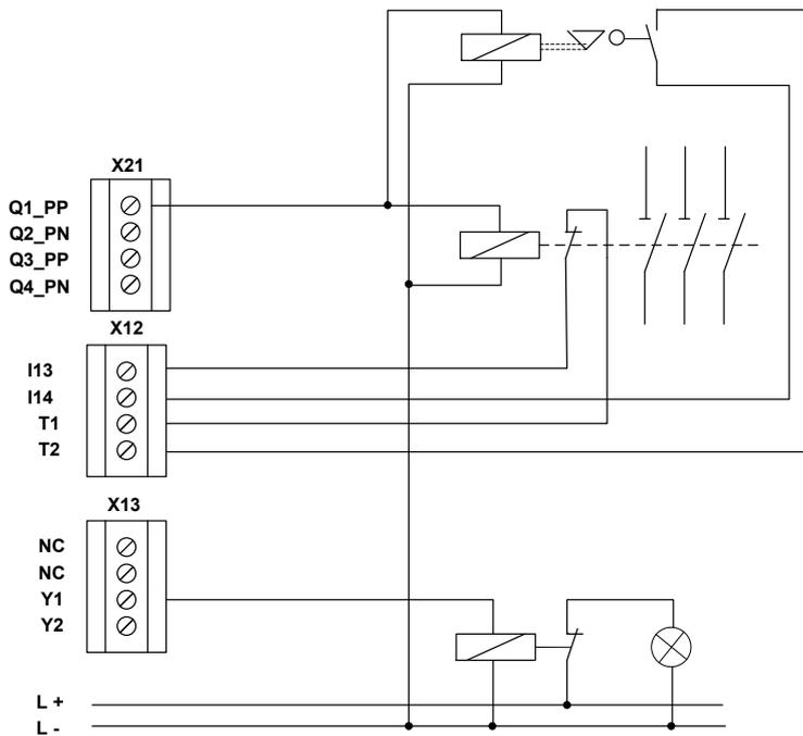
**Fig. 23: Single-channel switching output Q1\_PP with dual-channel external circuit as combination of electro-mechanical element and hydraulic/pneumatic valve and monitoring at two inputs**
