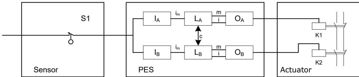
**Fig. 5: Single channel input element and dual channel processing with low to medium DC by signal processing in two channels and diagnose by means of cyclic testing, PI / SIL depending on permissible fault exclusions and test rate for input element.**
