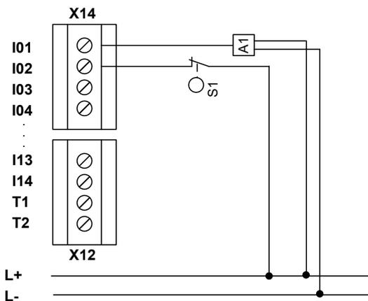
**Fig. 9: dual-channel input element heterogeneous, without cycling**
