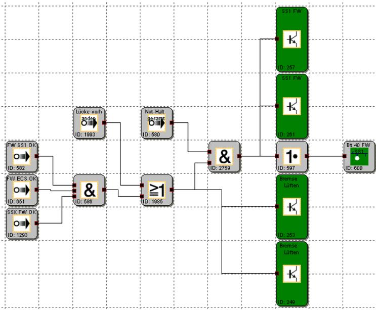
The carriage is switched off via two outputs (IQQ1.5 ID 257 and 1.6 ID 261).
