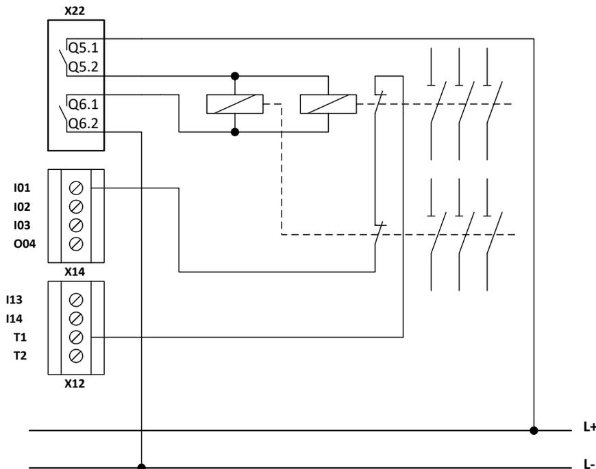
**Fig. 24: Two-channel switching relay output with external monitoring – group feedback**
