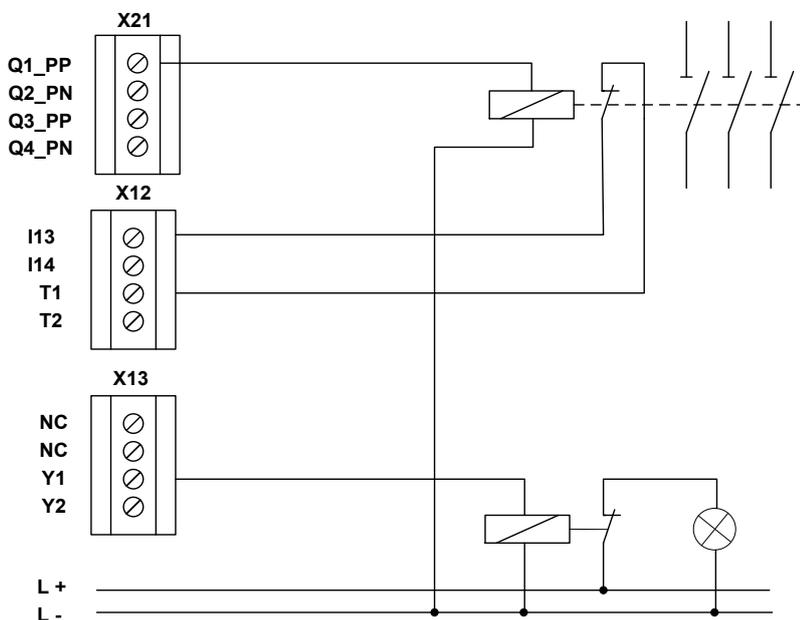
**Fig. 21: Single-channel switching relay output with testing**
