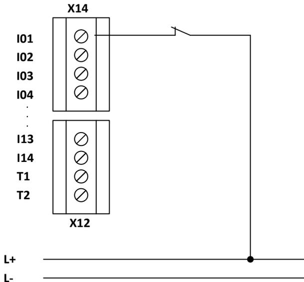
**Fig. 6: Single-channel, without cross-shorting test**
