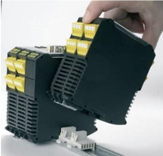
Insert the module from the top at an angle
