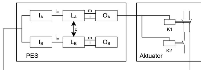
**Fig. 14: Single-channel output SMX (Rel 1 / 2, DO 0/1P, DO 0/1M) and dual-channel actuator with at least single-channel diagnostics**
