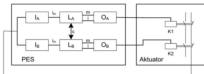
**Fig. 18: Dual-channel output SMX and dual-channel actuator with dual-channel diagnose**
