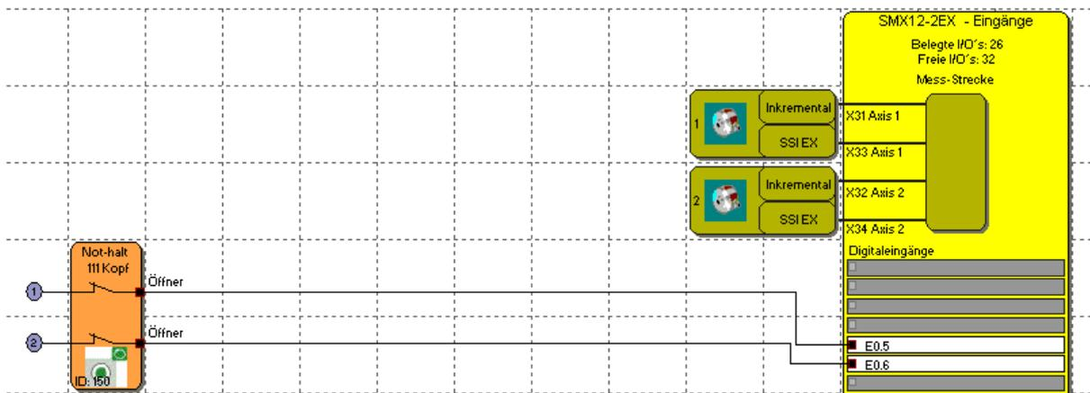
**Fig. 32: Emergency stop contacts from emergency stop relay with pulsing from the SMX**
