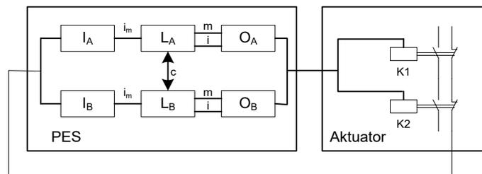
**Fig. 16: Single-channel output SMX with internal dual-channel processing (IQQx) and dual-channel actuator with dual-channel diagnose**
