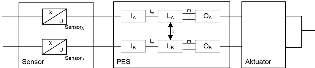
**Fig. 11: Dual-channel sensor system with separate signal processing in two channels, diagnostic by cross-comparison in the PES**
