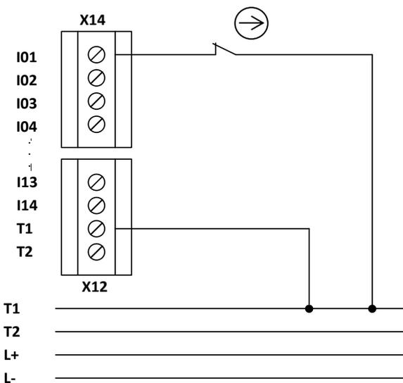
**Fig. 7: Single-channel sensor with cycling**
