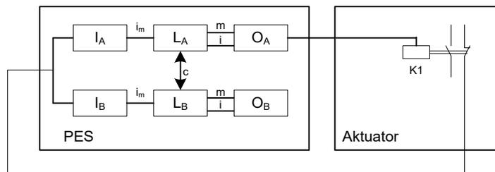
**Fig. 13: Single-channel output SMX and single-channel actuator with diagnostics**
