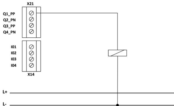
**Fig. 19: Single-channel switchingp-output**
