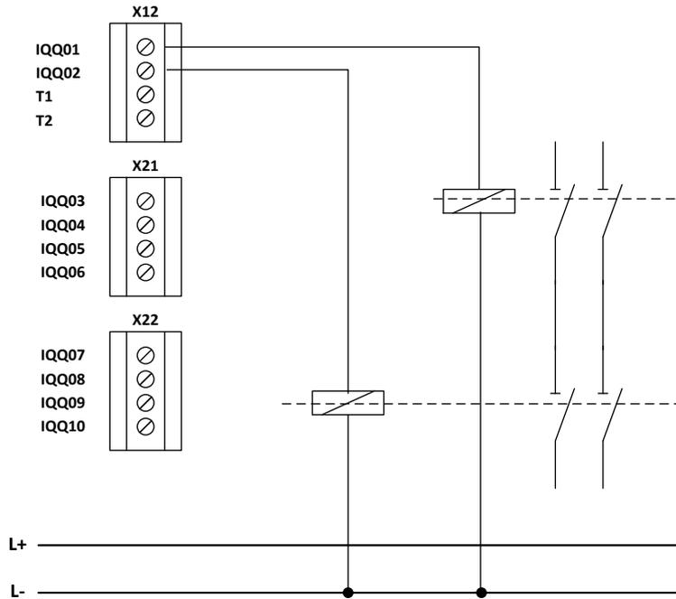
**Fig. 30: Redundant dual-channel outputs in the same group in conjunction with dual-channel switch-off circuit**
