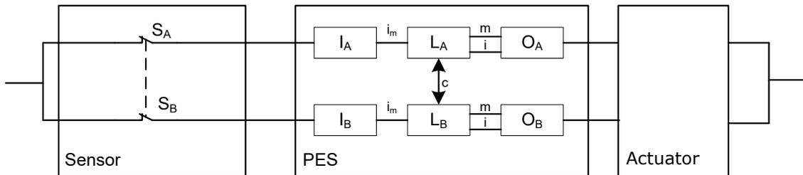
**Fig. 3: Two-channel input element in parallel connection (Cat. fault tolerance 1) with high DC caused by signal in two channels and diagnose by means of cross-comparison in the PES**
