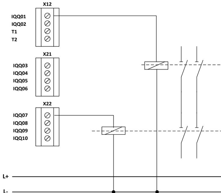
**Fig. 31: Redundant dual-channel outputs in different groups in conjunction with dual-channel switch-off circuit**
