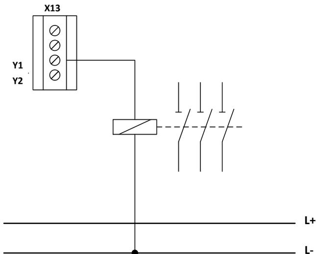
**Fig. 25: Wiring of a notification output**
