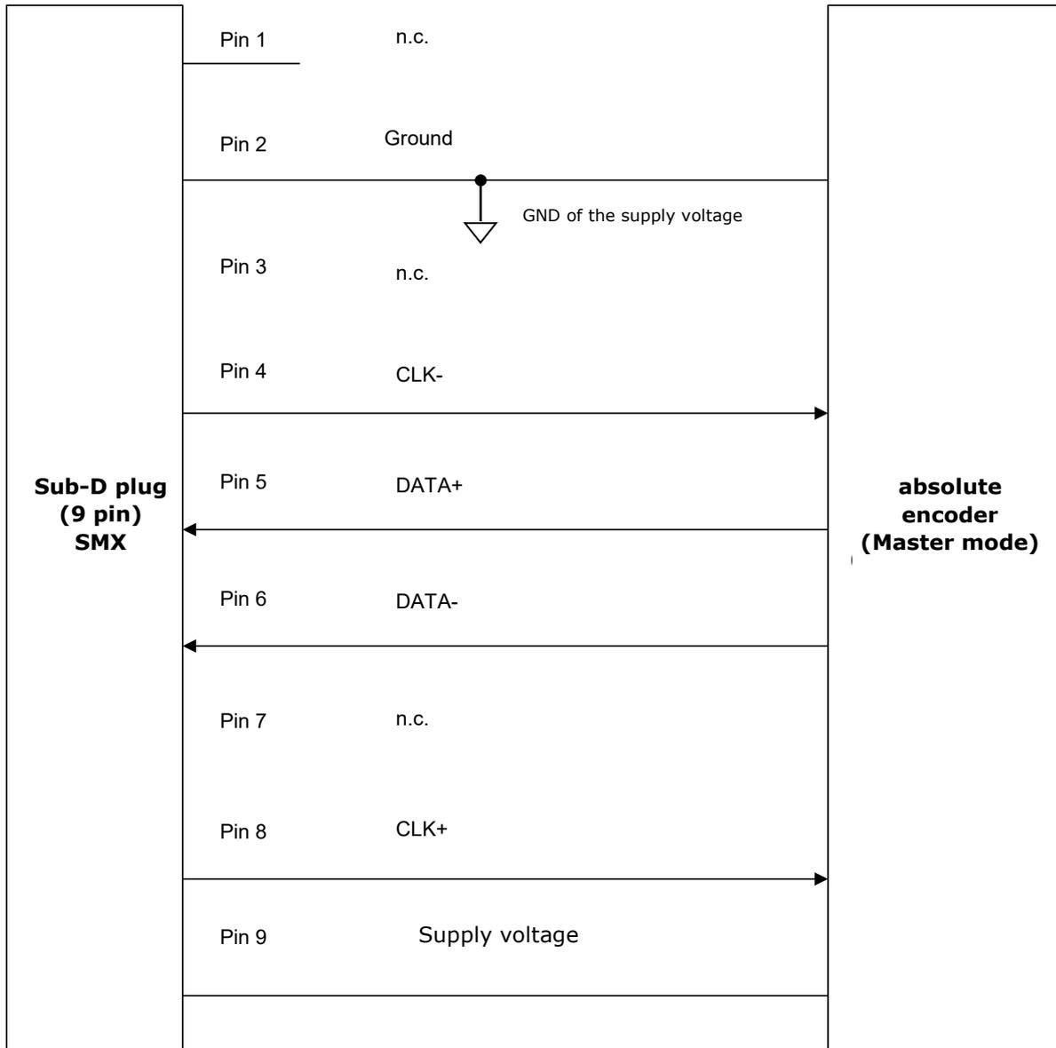
B With this type of the connection the clock pulses of the module SMX run to the absolute encoder and the data from the encoder to the SMX.
