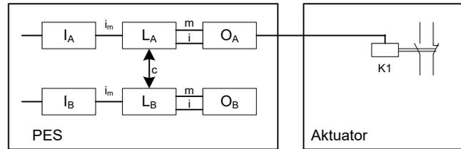
**Fig. 12: Single-channel output SMX and single-channel actuator without diagnostics**
