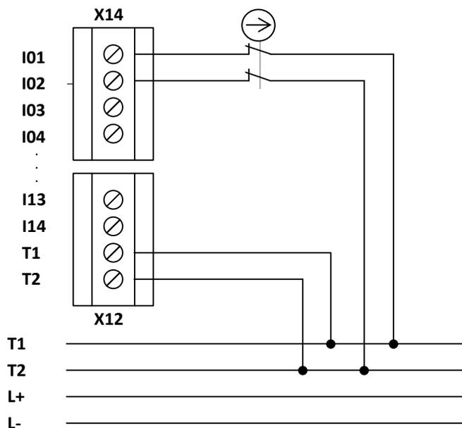
**Fig. 10: Dual-channel sensor homogenous with clock**
