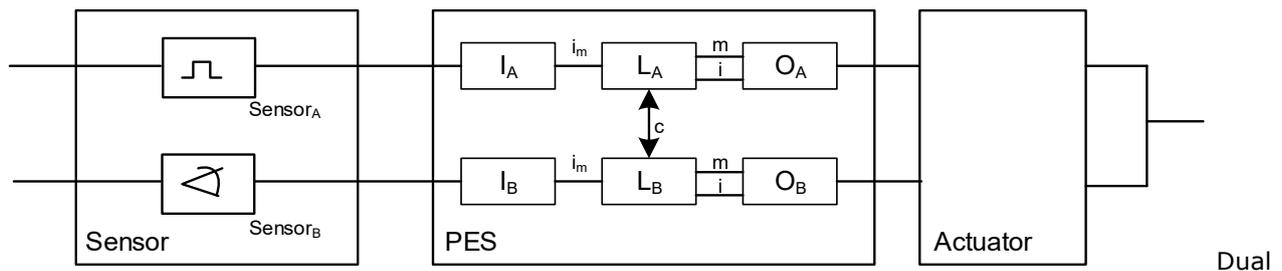
sensor system with separate signal processing in two channels, diagnose by cross-comparison in the PES
