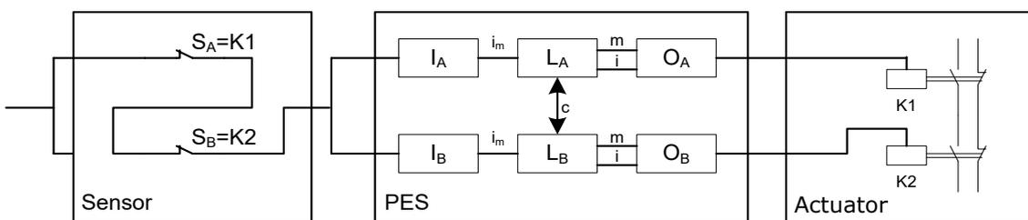
**Fig. 4: Two-channel input element in series connection (Cat. 4, fault tolerance 1) with low to medium DC caused by signal processing in two channels and diagnose by means of cyclic testing**
