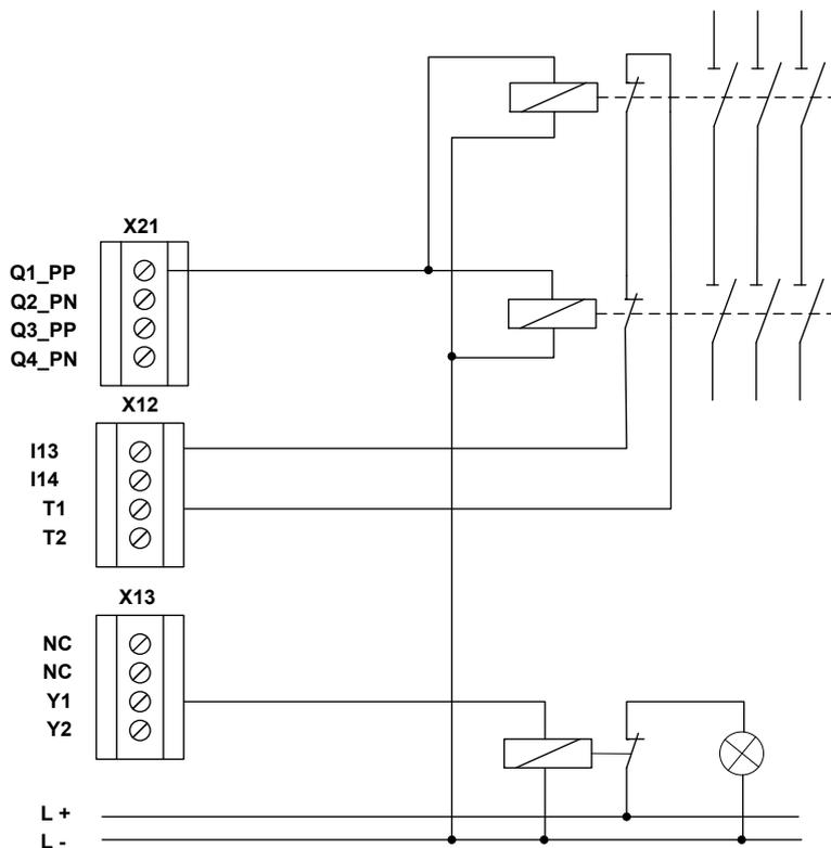
**Fig. 22: Single-channel switching output Q1\_PP with dual-channel external circuit and monitoring at output 13.1 as group feedback**
