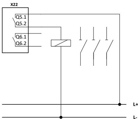
**Fig. 20: Single-channel switching relay output.**
