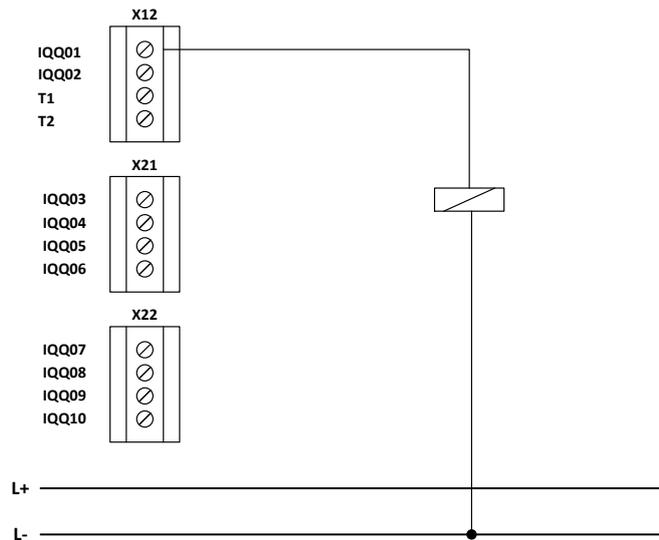
Fig. 26: Two-channel output with single-channel wiring without testing
