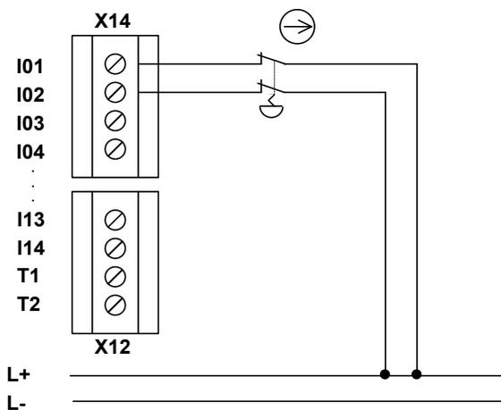
**Fig. 8: Dual-channel sensor homogeneous without testing, with positive disconnection**
