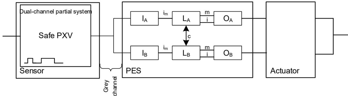
Sensor system with two-channel subsystem. Diagnosis through separate signal processing in two channels and cross-comparison in the PES as well as other specific diagnoses.
