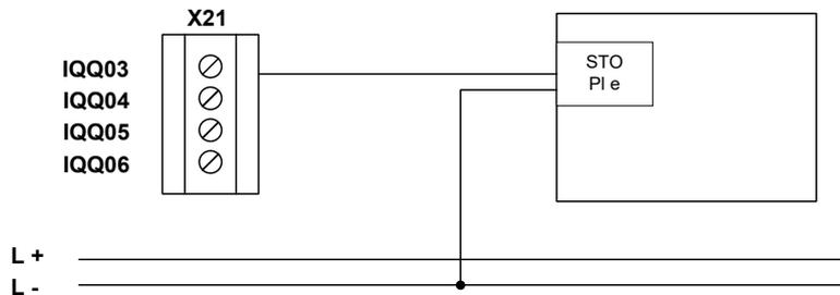
**Fig. 28: Dual-channel output in conjunction with device with tested switch-off**
