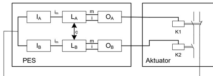
**Fig. 17: Dual-channel output SMX and dual-channel actuator with single-channel diagnose**
