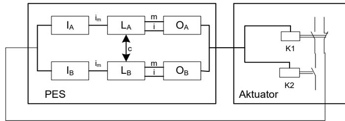
**Fig. 15: Single-channel output SMX with internal dual-channel processing (IQQx) and dual-channel actuator with at least single-channel diagnose**
